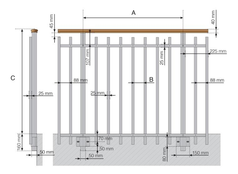
A - The c/c dimensions of the posts depend on the length of the sides and the number of sections
